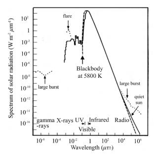
Figure 1.7 The measured spectrum of solar radiation (continuous line, with the contribution of bursts dotted), compared with the blackbody spectrum (1.4) (dashed).
