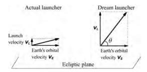
Figure 1.16 The difficulty of sending a spacecraft outside the ecliptic: because the Earth speed  $v_E$  is much greater than the launch speed  $v_L$ , the spacecraft velocity  $\mathbf{v}_L + \mathbf{v}_E$  in the solar frame makes a very small angle to the ecliptic.
