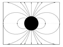
Figure 1.23 Magnetic field lines of a magnetic dipole aligned with the vertical axis. The black disc sketches the region (here the solar interior) where the currents producing magnetic fields are flowing.
