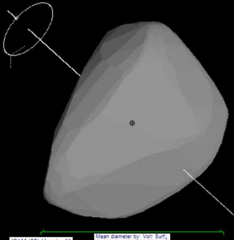
Black marker is centre of mass (assuming uniform density). The centre of figure is clearly located to the right of the marker.
