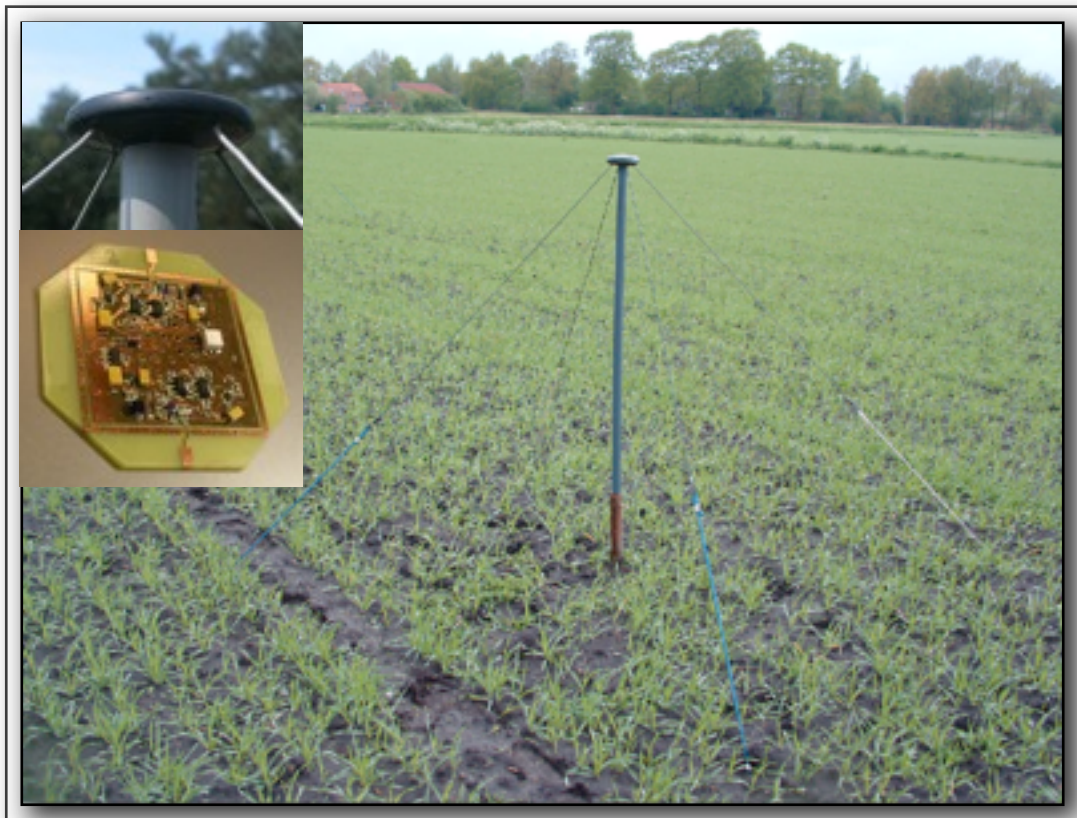
Low band antenna: 30 – 80 MHz 48/96 antennas/station
