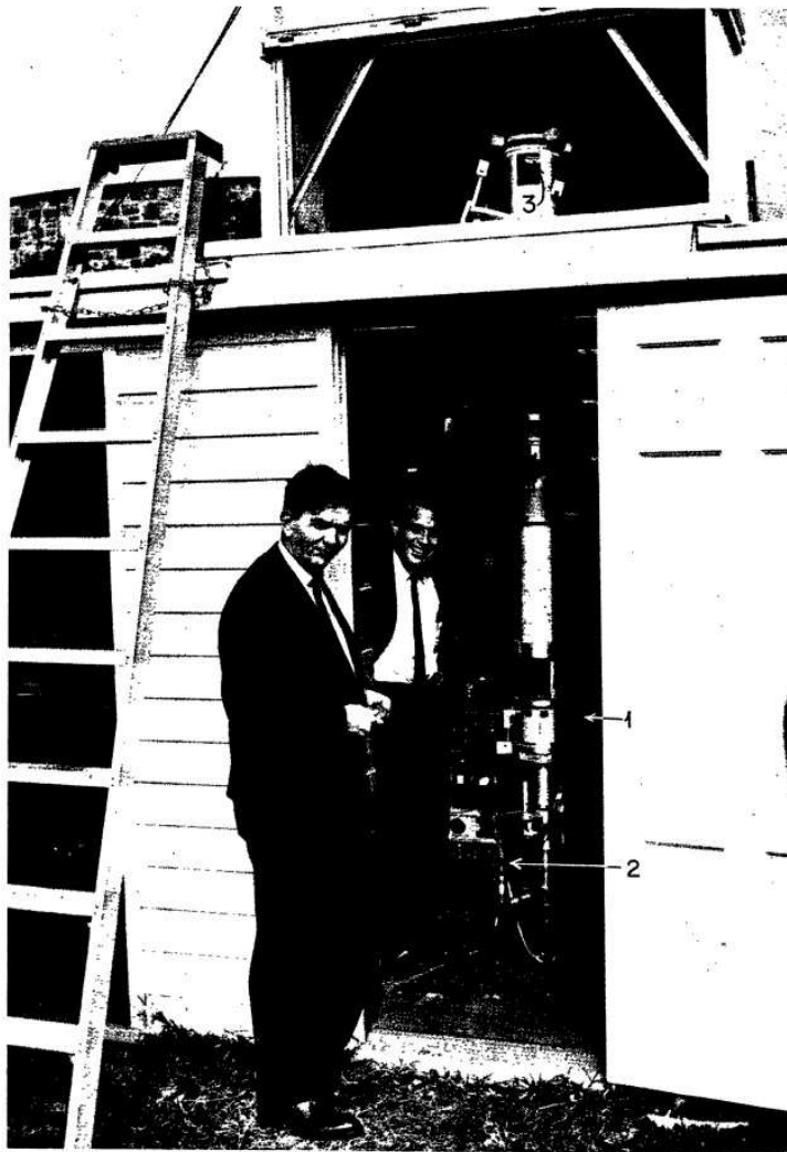
FIG. 29.—Telescope viewed from the front. The door (facing south) is normally closed when the instrument is operated. The rectangular observing port is 25^{\circ} \times 50^{\circ} . Parts shown: (1) Center photocell housing, (2) Viewing eyepiece, (3) Secondary mirror.
