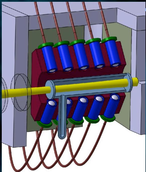
4 measurement channels for each spectrometer point
