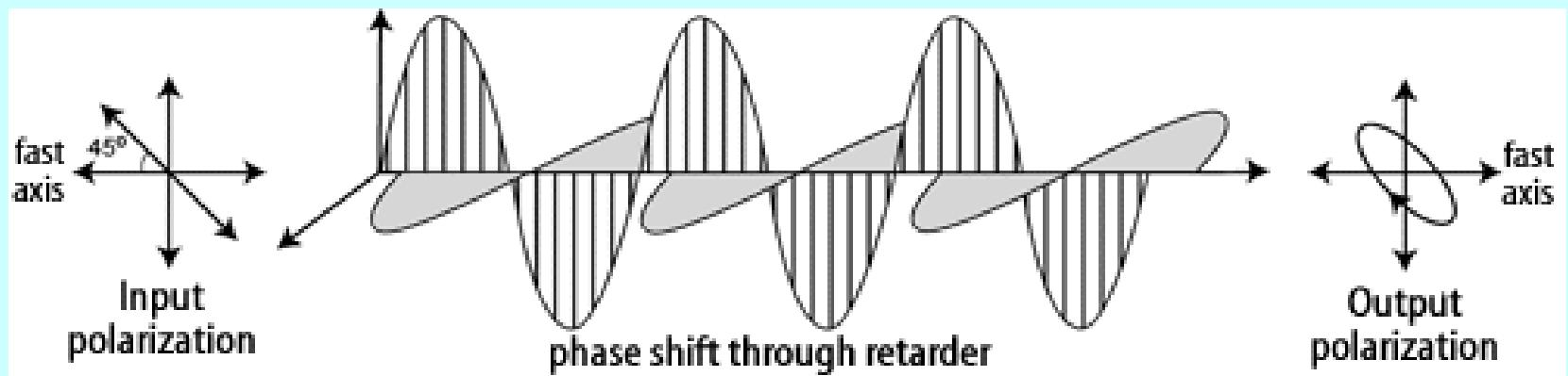
Create a phase delay between 2 beams
