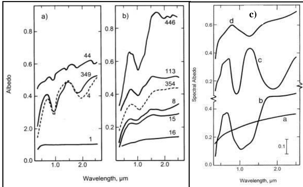
Left [a) e b)] spectra of asteroids compared with [c)] spectra of known minerals: a-iron-nichel, b-olivine, c-pyroxene, d-anorthite.
