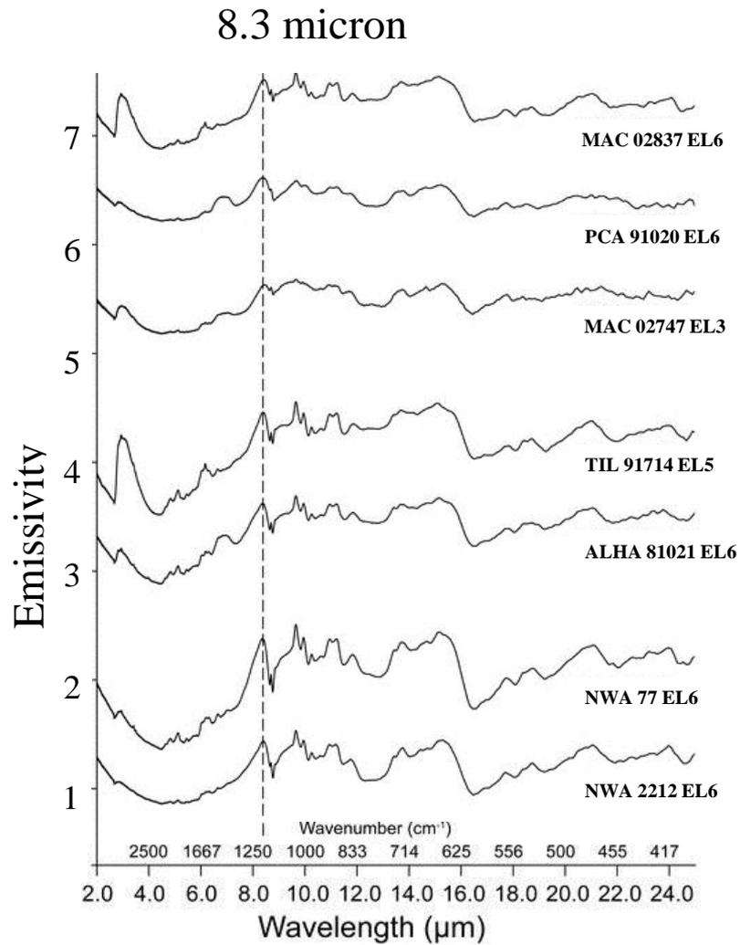
Emissivity spectra of enstatite chondrites
