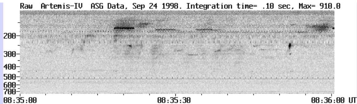
(a) Dynamic spectrum (flux) from sweep frequency receiver (ARTEMIS/ASG)
