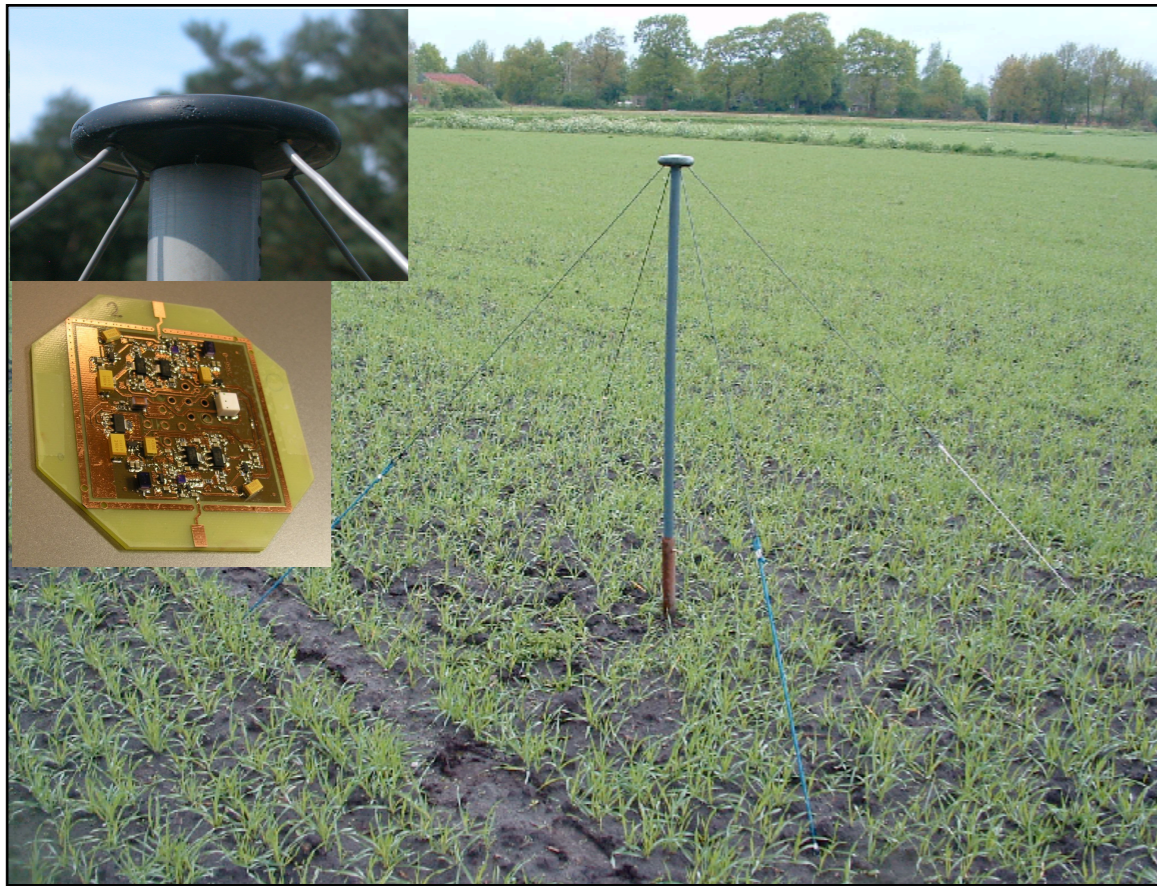
Low band antenna: 30 – 80 MHz 48/96 antennas per station
