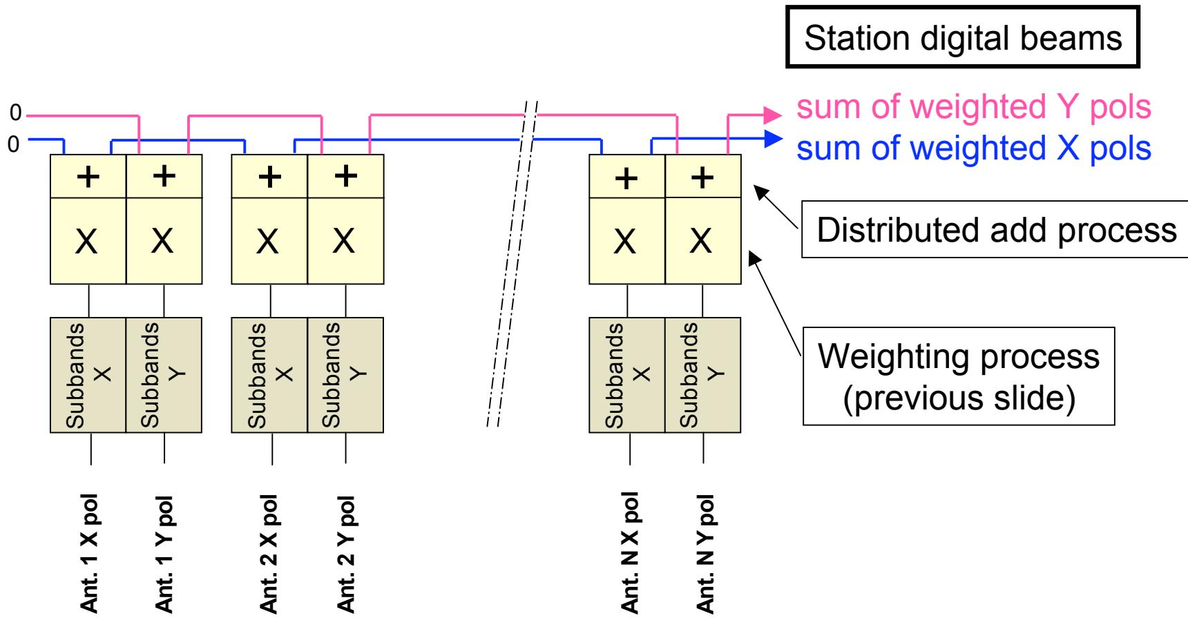
Digital beam = sum of all phase shifted antenna data to point at source position ( $\theta, \Phi$ )
