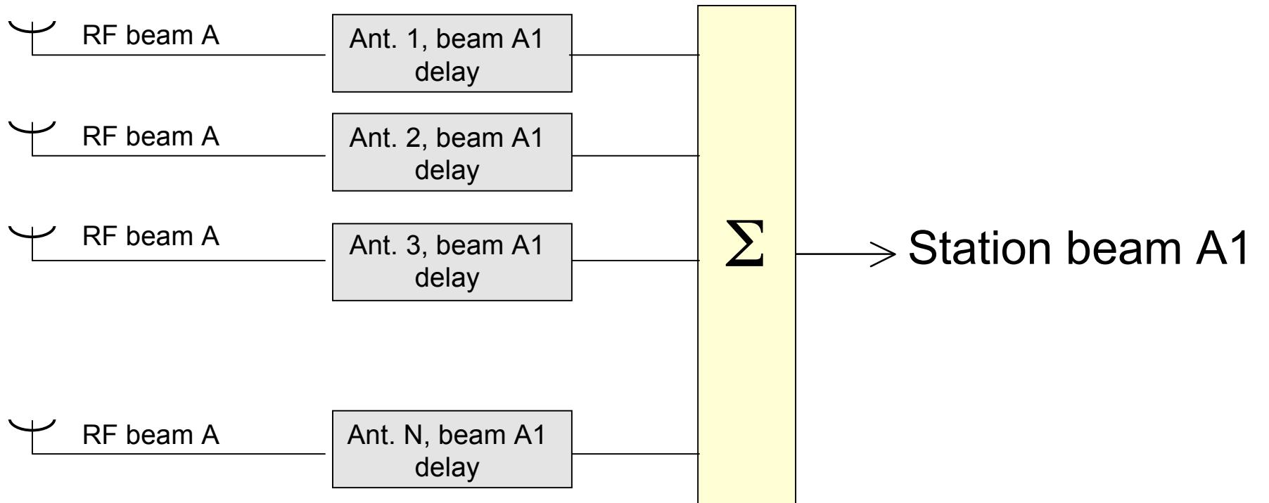
For k station beams (A1 to Ak): k-fold duplicate of the sum of delays
