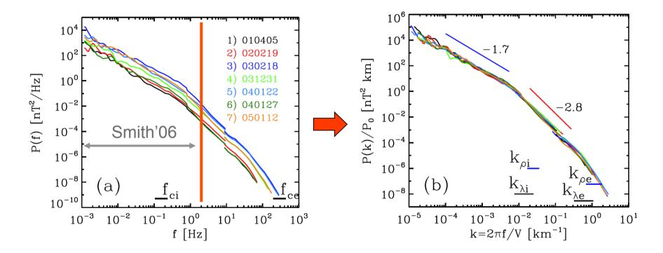
Superposition of different spectra gives one clear spectrum with 2 inertial ranges  $\sim k^{-5/3}$ ,  $k^{-2.8}$  (and dissipation at electron scales?)
