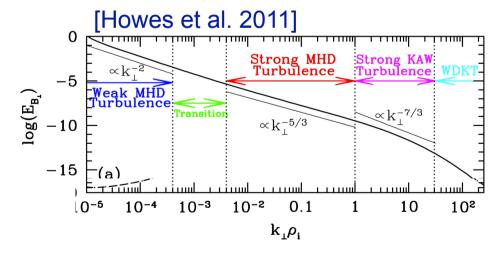
Cascade model with  $\sim k^2$ damping term (dissipation via linear Landau damping of KAW's) [Howes et al. 2006, 2011]
