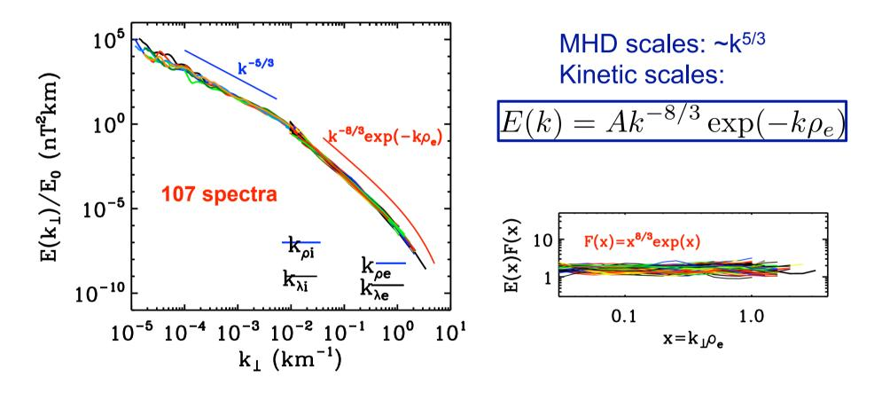
Compensated spectra are flat at  $k\rho_e > 0.03$  and for ~2 decades in scales => the model describes well all observed spectra.
